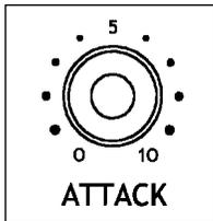
The attack knob controls the amount of time it takes the output voltage to reach the maximum level once the gate is initialised.
