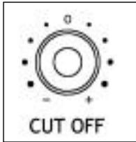
The Cut-off knob controls the point at which attenuation begins. Frequencies above the cut-off point are attenuated at 24dB/oct.
