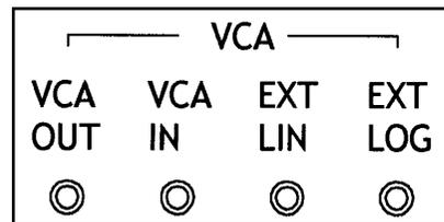
The VCA is an amplifier which allows its gain to be altered by a control voltage. The VCA within the MARS has both logarithmic and linear controls creating unique contours.
