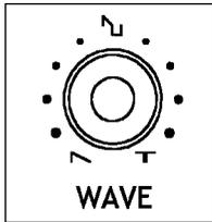
The wave knob controls the initial wave shape from the VCO. In the anti-clockwise position a saw tooth is generated, in the clockwise position a pulse is generated, between the two positions the wave shape alters from sawtooth through various sawtooth/squarewaves to a 2% pulse. The waveform is fully variable with no fixed point.
