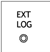
This input allows logarithmic modulation of the VCA by an external source.
