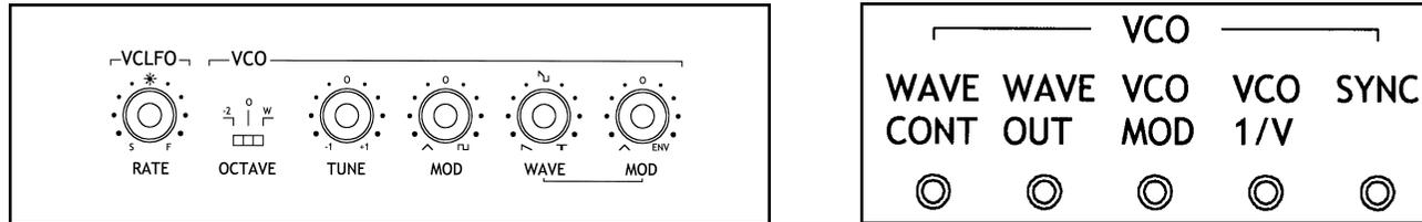
The VCO is the primary sound source within the MARS. It creates the raw waveform which is then processed and modified by the other synthesizer circuits.
