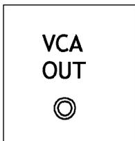
This is the output of the VCA, it is also the final output when used as a complete synthesizer.
