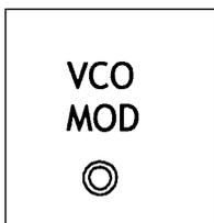
This is similar to the VCO 1/V input but should be used for external modulation, (eg: LFO, sample and hold, ENV).
