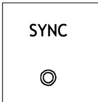
This is a hard sync input used to reset the VCO waveform using a second oscillator. A wide range of frequencies, waveshapes and levels will determine the type of sync generated.
