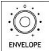
The envelope knob alters the cut-off point according to the set up of the envelope generator allowing automated shaping of the filter negatively and positively.
