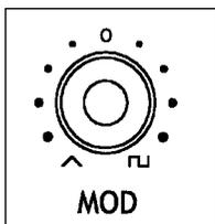
The Modulation knob introduces either triangle, square or no modulation to the oscillators frequency (a maximum of two octaves, from the VCLFO).
