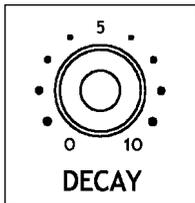
The decay knob controls the amount of time it takes the output voltage to fall to the sustain level once the attack phase is complete, providing the gate has not already ended.
