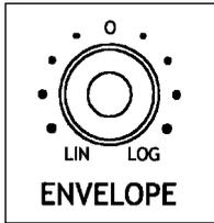
The envelope knob sets the amount of voltage controlled amplification from the envelope generator. Linear and logarithmic control is available giving unique and unusual amplification contours.
