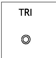
This output gives a triangle wave output of +/-5 volts
