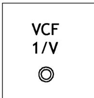
This is the main control voltage input for the VCF and has characteristics of one volt per octave. This should be used as your main control input from a keyboard/ controller.
