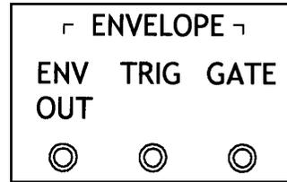
The ENV is a method of generating a control voltage, the waveshape is created in 4 stages: Attack, Decay, Sustain and Release which can be adjusted individually. The output of the ENV can control any voltage controlled input.
