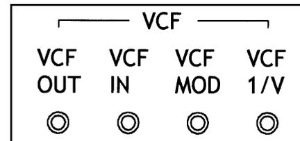
The VCF is a low pass 24dB/oct ladder filter, it has the ability to attenuate/eliminate frequencies above the cut-off point. This type of filter can create sounds associated with classic American analogue synthesizers.
