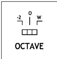
1. In the '-2' position the tune knob controls the initial frequency of 32Hz by +/- one octave.
