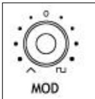
The mod knob introduces either triangle, square (from the VCFLO) or no modulation to the VCF's cut-off point.
