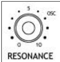
Resonance is used to accentuate frequencies around the cut-off point, as the resonances increase the filter will begin to ring and will self oscillate at high resonate settings producing a sine wave (the frequency of which is controlled by the cut-off knob).
