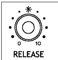
The release knob controls the amount of time it takes the output voltage to fall to '0' once the gate has ended.
