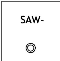
This output gives a negative sawtooth with an output voltage of +/-5 volts.
