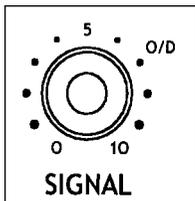
The signal knob controls the audio signal level coming from the VCF into the VCA. The VCA may be over-driven (clipped) in the range of 5 - 10.
