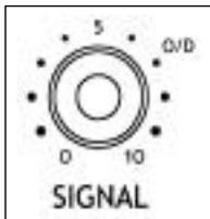
This signal knob controls the audio signal level coming from the VCO into the VCF. The filter may be over-driven in the range of 5 - 10.
