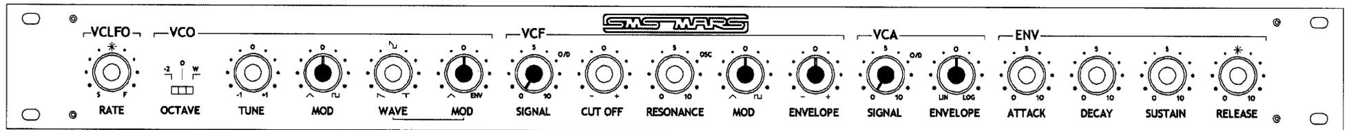
WITH THE HIGHLIGHTED CONTROLS IN THE POSITIONS SHOWN, THERE ARE NO INTERNAL SIGNAL OR MODULATION ROUTES.
