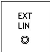
This input allows linear modulation of the VCA by an external source ( the usual control input from an envelope generator).
