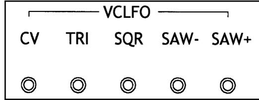
The VCLFO is a wide range oscillator used to modulate control inputs, eg: used for vibrato, tremolo and trill. It is internally routed to the VCO and VCF (see INTERNAL SIGNAL ROUTE page 3).
